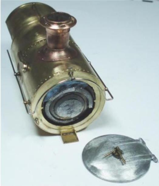
Here is the rebuilt smoke box fitted with half a pound of rolled lead and fixed in with blue-tack. I was taking no chances with it this time however, it has been suggested by (I think) Bob Alderman, that liquid lead and a resin based powered glue is non-reactive.
