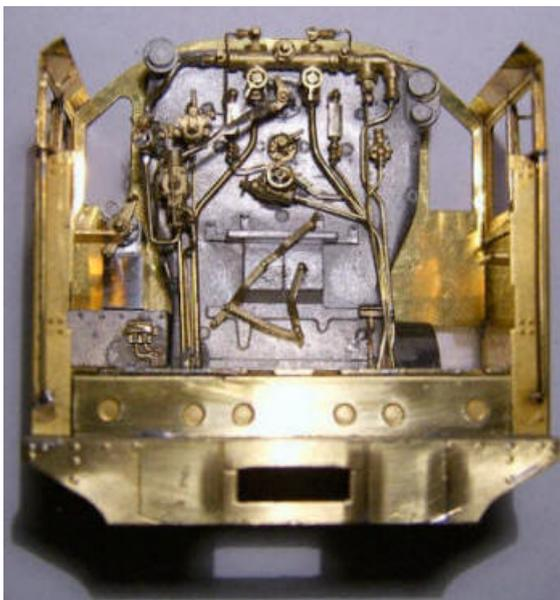
The back head and reversing gear mocked up in the cab. They will be fitted after the painter had completed his work. This represents a satisfying couple of afternoon's work identifying where all the pipe runs go from the diagrams and various pictures, none of which matched! So much for standardisation of the original.
