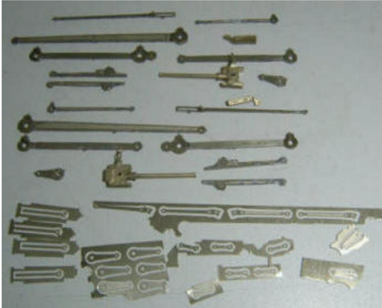
The next job is the motion, shewn here with some of the laminates partly soldered up and awaiting cleaning and polishing. So this is the "before" picture. Notice how short the slide bars are, of which, more anon.
