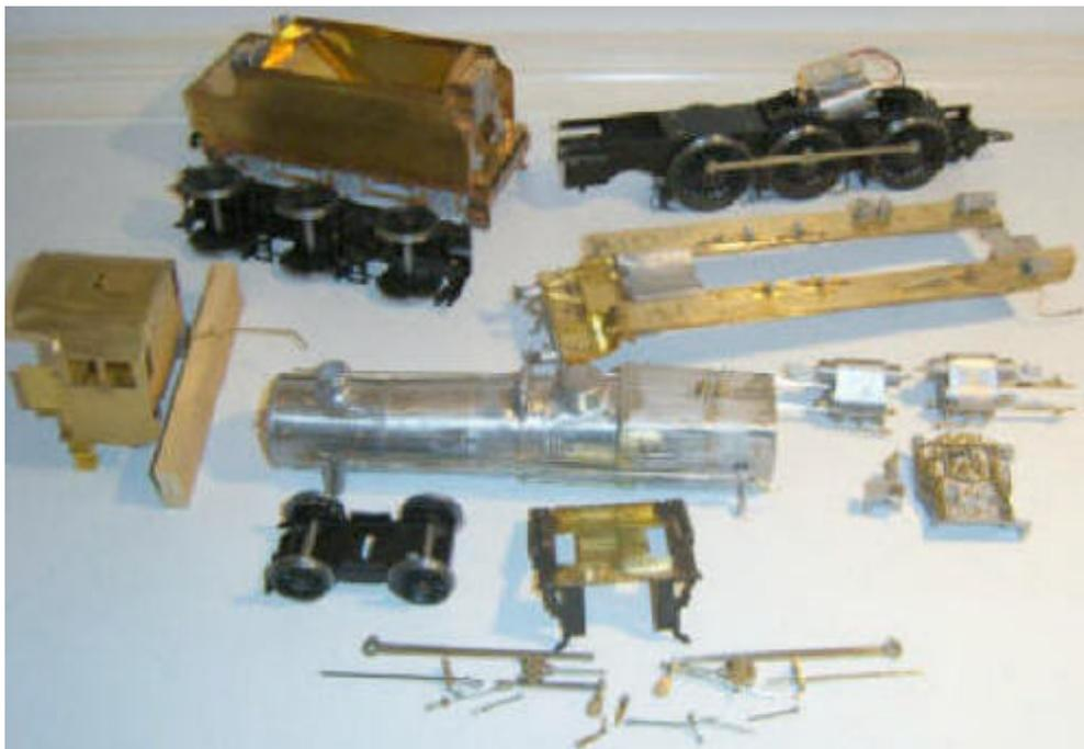
Not easy to solder to a huge lump of white metal either (I destroyed one and had to get replacements) so I used old fashioned Araldite baked in a coolish oven overnight. I think the bars should have gone the full length of the cylinders for strength. So that they would not have to bear any appreciable load, I lined the cylinders with brass tube to take the piston
