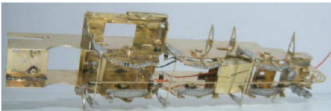
The chassis on its wheels with the motor temporarily fitted but awaiting installation of the cylinders. Later would be added sandboxes and sundry other pipe work and fittings.
