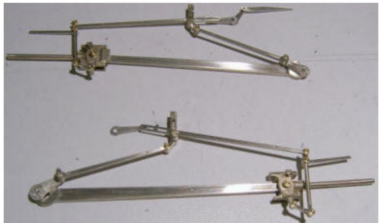
Personally I would rather that casting such as these came with holes (possibly even ready tapped, say, 8BA) for the rod to be fitted. Cast rods are frequently not as round as they might be and are often bent out of shape too. Good nickel silver rod would be both straight and round.
