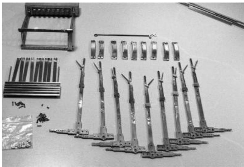
Important too to remember that the block must continue to move easily once the lever has been painted. The lift arm is soldered inside this and the short angle at the base trimmed to size.
