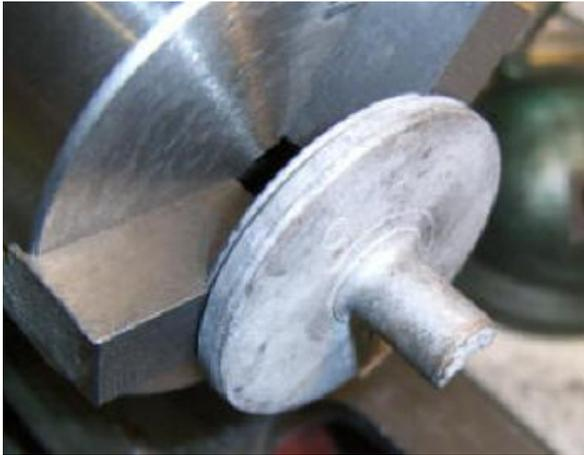
The first thing to do is set the casting up in a set of soft jaws by its tread, having first filed off any casting pimples and true up the spigot and the back of the wheel. The soft jaws are turned down to be a slightly larger diameter than the wheel itself. This provides more grip and a very positive location. Mark each wheel to indicate jaw 3 (or whichever is convenient for you).
