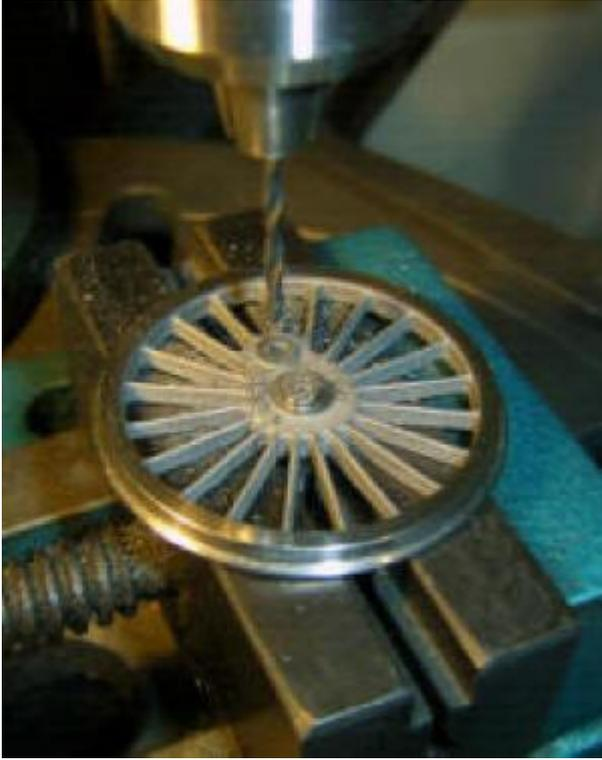
Insulation is achieved by turning up paxolin bushes for one side, or cutting alternate spokes, filling with araldite and repeating the remainder when the glue has cured.
