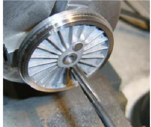
The spigot is then sawn off while mounted in a vice and remounted in the chuck by the tread using the soft jaws again, ensuring that the mark is now back on jaw three.
