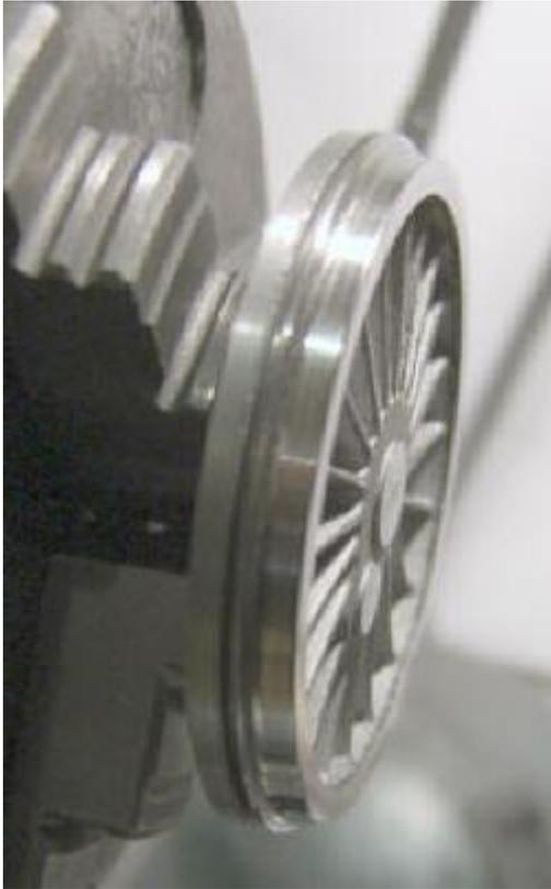
The flange and tread are then turned down to exact size using a forming tool. I use a form tool from the Scale 7 Society who produce one for fine scale as well, which is sharpened prior to turning up each wheel.
