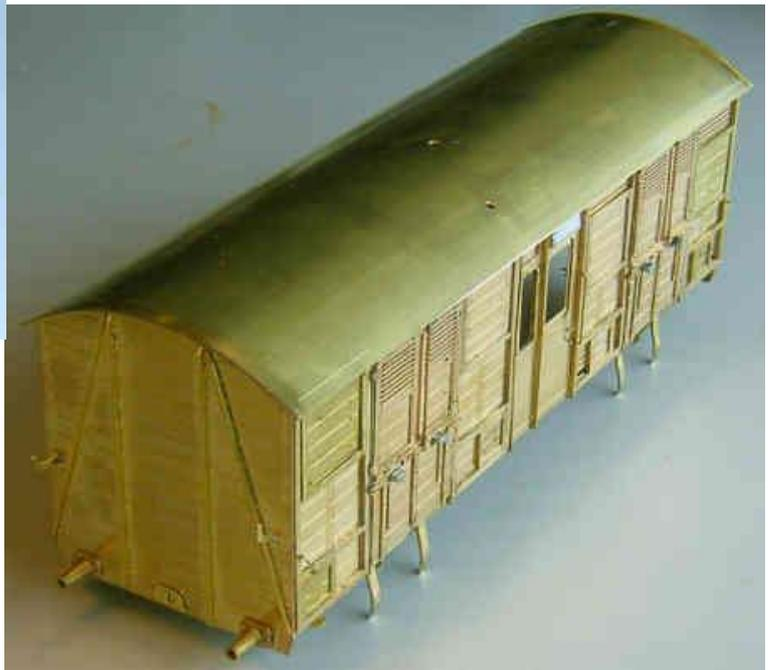
The roof needed soldering at the ends only. I tack soldered it at the centre from inside, there are convenient etched witness marks provided to ensure it is centered, checked for square and overhang and then seamed it up; an easy job with the RSU.
