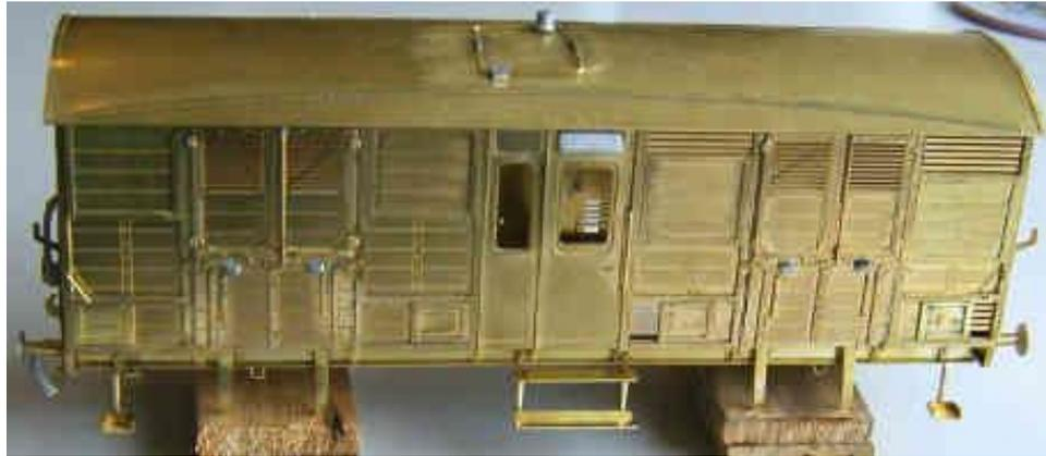
The completed body ready for the paint shop. The steps have been fitted using modified Slater's GWR step supports; this is just personal preference for stronger fittings. The method
