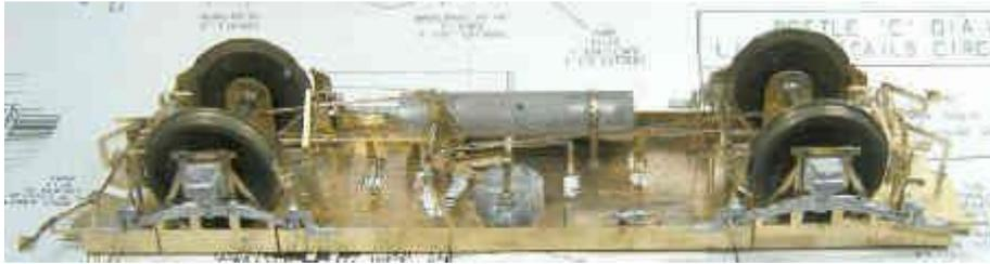
the under frame. All the levers, including that on the vacuum cylinder, operate. However, once the gear is all fitted it will be soldered solid.
