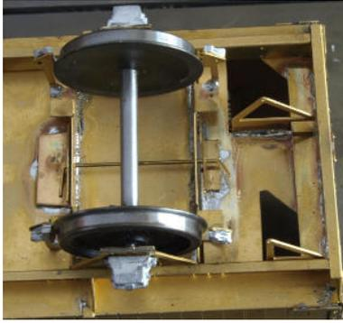
The original axle boxes were fine. However, what was not fine was the compensation unit which did not fit. The etched hole in the floor was too small and had to be opened out and one of the fold-up supports for the pivot wire had to be removed and a substitute scratched up. In this picture it can be seen that it will need to be moved again to prevent too much fore and aft movement.
