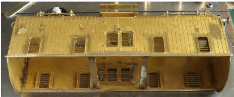
To prevent the sides bowing in, two cross pieces were soldered in just under roof level. The etched part
