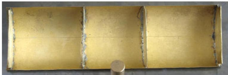
After cutting it to the correct width, which required a great deal of careful measurement, it was rolled to shape and the edges bent over to the vertical. It is such a small turn that even the hold and fold could not cope with it so I had to use pliers, not ideal.
