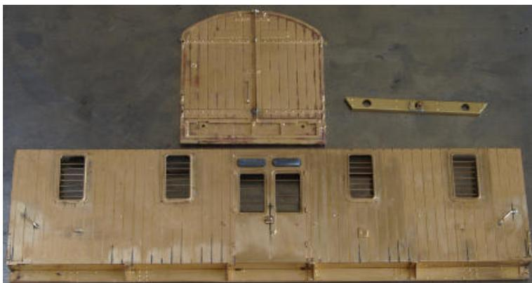
The sides and ends ready to be assembled. The diagonal hand rails at each end are not catered for so rather than drill holes, I flattened the ends of the rails and soldered them in place.
