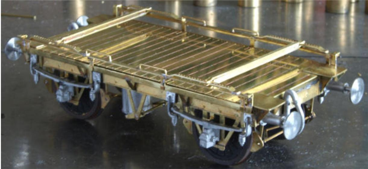
The restraining bars across the bed are designed to make up from several layers of etch but this time I used some 1.5mm square brass stock instead, much easier.
