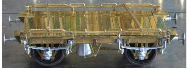
These three shots of the completed vehicle shew much of what the work is about in building the vehicle. The springs, hangers and axle boxes are all separate castings.
