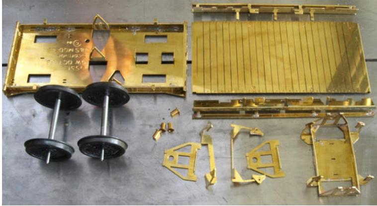
Here are the major parts ready for the main construction to commence. The basic floor is done together with the solebars and buffer beams. Building the basic underframe and detail is relatively easy; one simply has to dry run everything.
