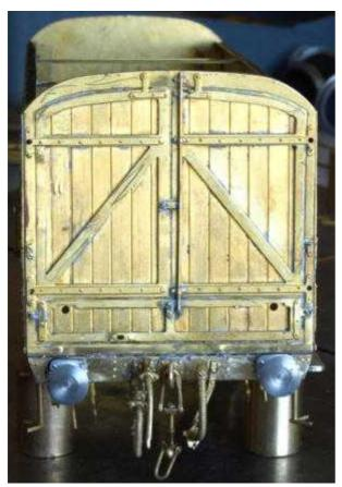
Now largely complete and awaiting some final parts fixing. The kit provided for sprung buffers using white metal housings and lost wax brass buffers to be sprung from behind with wire. The latter were very poorly cast (though again, from excellent masters) so they were scrapped and replaced with some internally sprung ones from Hayward.
