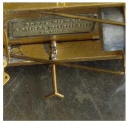
adequate but somewhat delicate in my view so I used Slater's step supports instead suitably modified by filing off the fixing pins and rivet heads, bending them straight and then fitting them through the etched holes in the sole bars, bending them up from behind and soldering in place.
