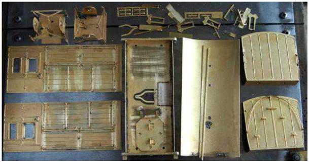
The rain strip on the roof is fitted in an etched groove, which needs to be opened out with a scrawker a little to make a good fit. It is easy and effective.
