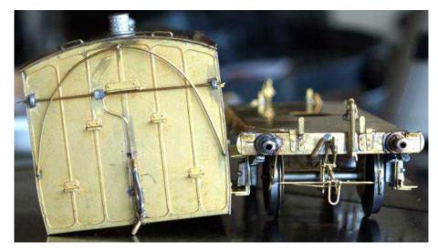
The vacuum and Westinghouse pipes were white metal and considered vulnerable, so they were changed for Slater's vacuum pipes with the base bent at about 40° to centre the pipe
