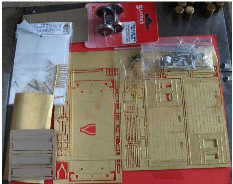
There are three sheets of instructions printed both sides; mostly captioned photographs of the vehicle under construction. There was also an over scale, dimensioned, drawing that proved most useful in identifying some parts and how it
