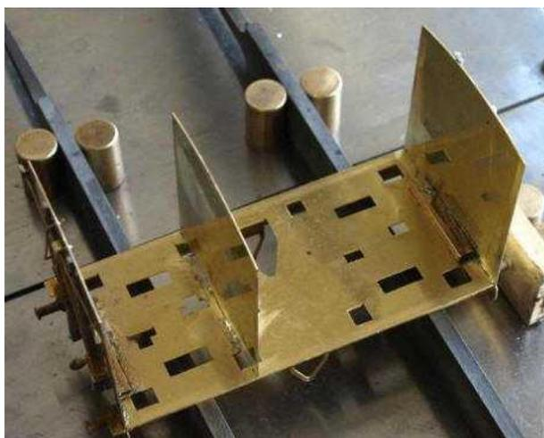
To fit the ends and compartment partition required a jig so that the floor could rest on its solebars. Some magnets and a couple of files on the steel plate did the trick. The one at the step was fitted first, then the partition and lastly the other end, that way there is always space to hold a small engineer's square to ensure a right angle.
