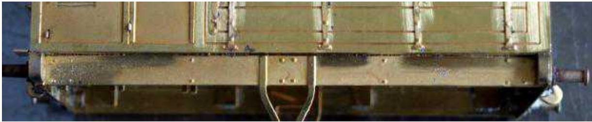
It was then a simple matter of soldering the parts in situ. A little fettling ensured they fitted the shape of each beam end correctly. It took a couple of hours but avoided messy fillers and the dusty process of cleaning them up once dry.
