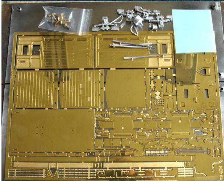
The kit, which used to be sold by MSC, arrives as a flat pack containing a sheet of hard, bright, etch attached to sheet of stout card, various castings in white metal and a set of Roxey lost wax buffers. These have brass shanks and heads so must be from an early
