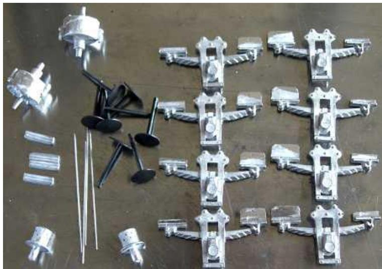
White metal parts ready now for fitting. The axle boxes and springs are interesting in that they slot over the edge of the solebar. Here they are cleaned up with part of the fixing flange cut away for the buffer shanks to operate.
