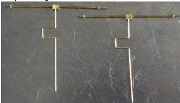
The alarm gear was made using some small scraps of brass and wire. The wings on the ends of the rod are made
