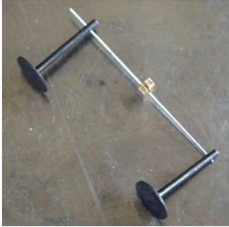
it to take the steel spring wire. Once the buffers are fitted together with the spring, the brass anchor is fitted and soldered in place thus. With care, it is possible to
