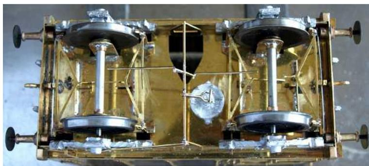
Meanwhile I have completed the underframe details, which are simple. Again, as for the large horseboxes, I omitted the details behind the wheels, as they are invisible in normal use.
