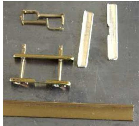
from brass angle and Slater's step board supports, which gave a more robust unit. The supports needed modifying to allow for narrower step boards and the removal of the fixing pins; the steps were then soldered in place on the solebar
