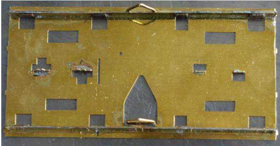
The floor with parts fitted for the solebars. These have small ninety-degree turnovers at each end however; they need to be removed, as they will foul the buffer body shanks, which are
