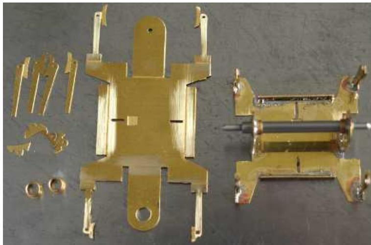
The time came to begin fitting the wheel sets, one of which is a rocking set to compensate the vehicle. The trucks go together quite well the only difficult bit being opening out the tiny holes in the wheel bearing supports, a longish job with broaches. The compensated truck is
