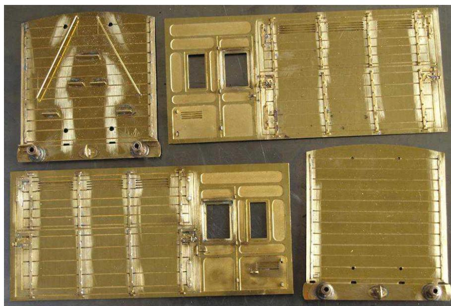
As is my usual practice, I fitted as many parts as possible while the sides and ends were still flat. The door handles came from a set of Slater's lost wax castings. The handrails on the step end were measured from the drawing and
