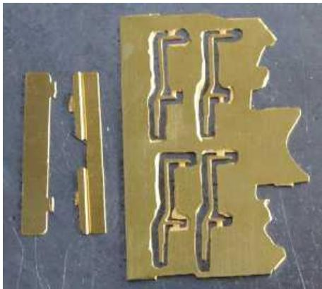
The steps proved to be 'interesting', the etch includes parts for the step supports as shewn here. They are designed to be laminated in pairs but in my opinion, would be far too fragile. Further investigation revealed that the flat of the step boards were a scale 4" wide while the drawing indicated they should be 8" and, as a single layer, I deemed them far too thin. I scrapped them and decided to scratch some up
