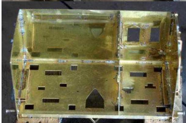
Once the ends were tacked in place and checked a substantial piece of rectangular brass tube was soldered into the join to strengthen it.
