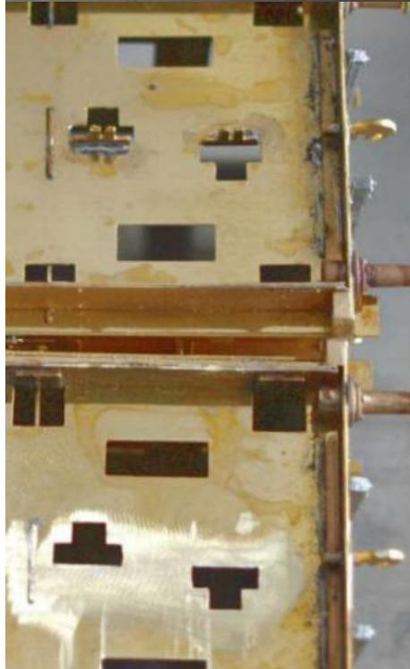
designed with two slots in the housing to fit over fold up tabs under the floor.
