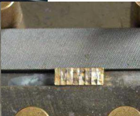
thickness is to use Milliput; I do not like the stuff and think it fiddlier than making some brass inserts. I cut eight pieces of 2x6mm brass
