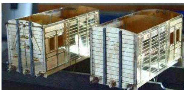
Finally, two bodies ready for fitting the underframe and roof.
