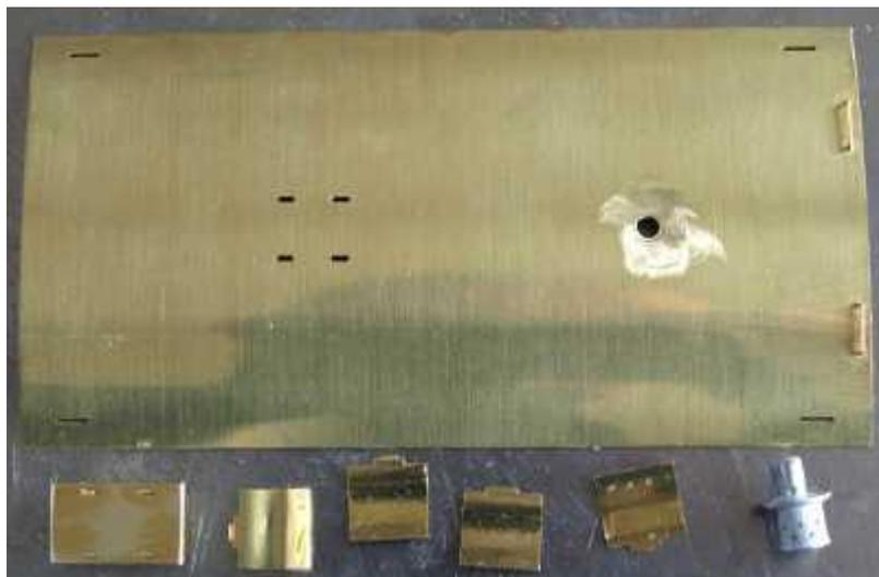
The roof is designed to be removable with tabs provided that are soldered into slots in the roof corners. They work well though I had to cut a few corners out to allow for the strengthening parts I had fitted in the body corners. The ventilator is made up from five parts that fit well and
