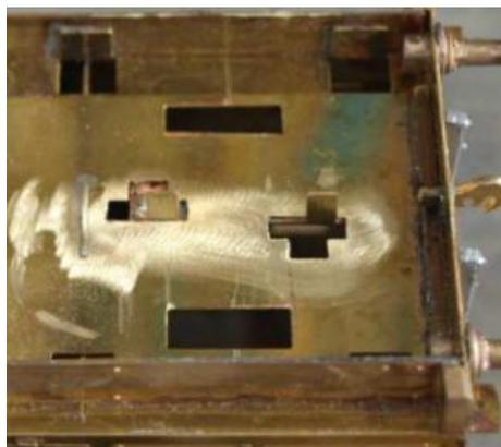
I removed the pivots as in the picture above right and filed the edges where they had been to line up on the centre line of the floor. Then made a new pair
