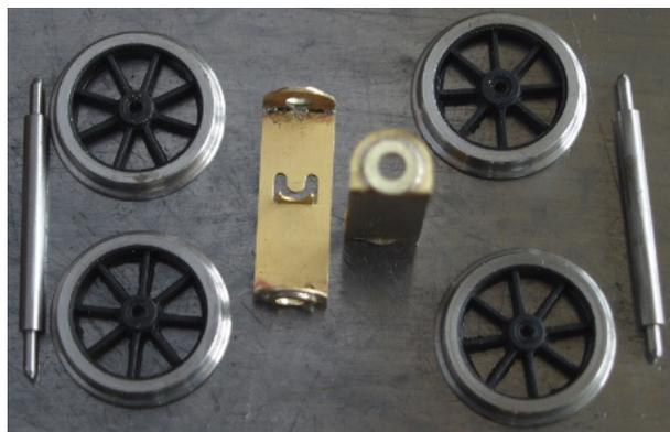
The wheel units are not of the type usually found in WEP kits; there is not room for them so a slightly different method is used. The rocking axle pivots about the central pillar with oval holes in the supports. I do not like single thickness bearings and so laminated some brass washers in place and opened the holes in the compensated unit to
