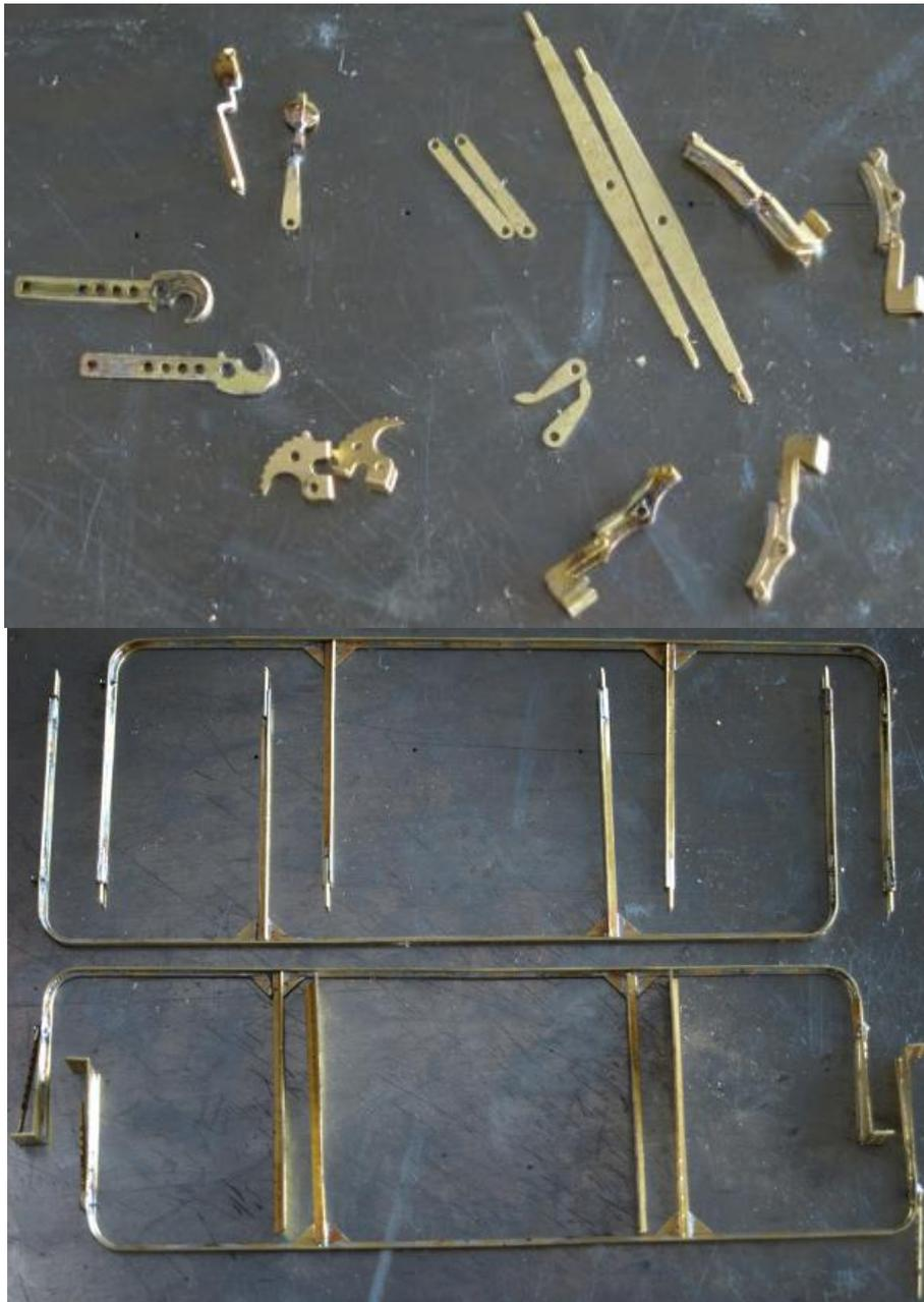
Here are most of the parts for the brakes; the blocks and hangers must be fitted to the body before assembly has progressed very far. They fit to inside side sheets for the wheel covers; I fixed them to the parts (one in each corner in the first picture) before fitting those parts to the body. The frames that hold the crates upright were made up largely as suggested except that I decided to make the locking bars movable and the non-fixed frame removable too.
