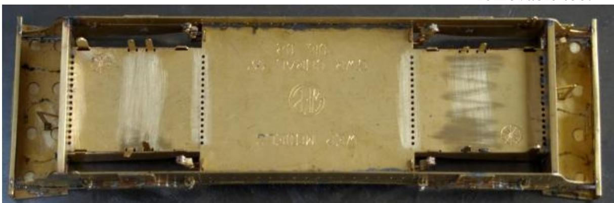
The frames need care to get the angle iron accurately soldered. This is an edge solder at right angles to the flat side. The rare earth magnets came in very
