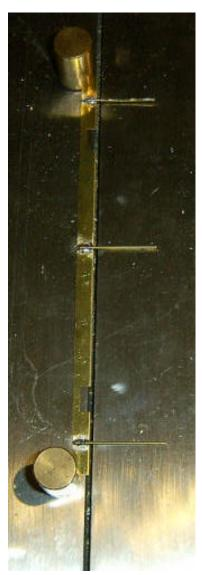
twisting the tabs at the rear. The method is easily visible in the back view of one side and end. All the parts that can be fitted while still "in the flat" have been, including lamp irons. All that remains to be fitted on the body after assembly are the handrails.
