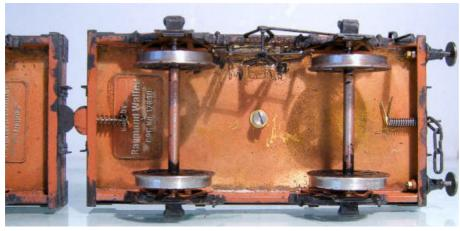
Very simple and uncomplicated; a piece of brass strip, bent over at 90° on the left and then sprung with a small cotter pin at the other. KISS - keep it short and simple.
