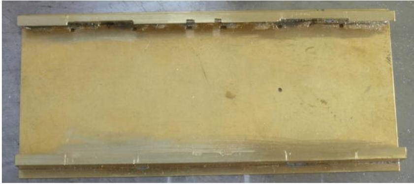
Here is the floor before the ends and sides were fitted and you can see that several cut outs were necessary for the axle guards and V hangers to fit
