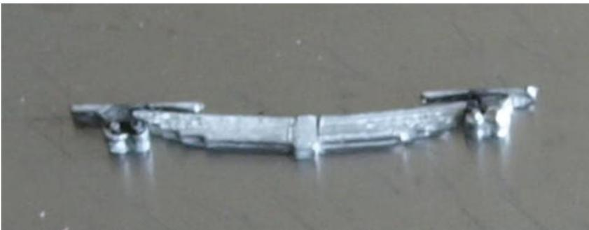
The springs and hangers come as separate items and clearly are intended to be fixed inside the sole bars. Unfortunately, this is not possible due to the W irons being in the way. I used Loctite 408 to fix the springs
