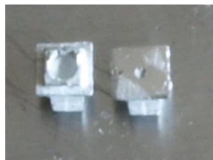
The axle boxes also need to have their backs filed down flush to be fixed to the W irons. Here, the three parts have been fitted to vehicle.
