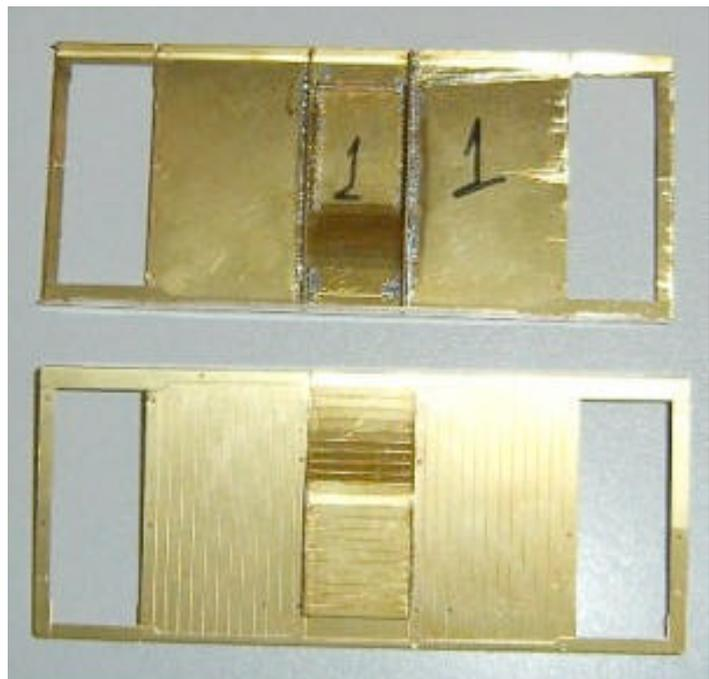
The tabs at top and bottom locate the part easily. Carefully solder from the inside, including the overlap at the bottom.
